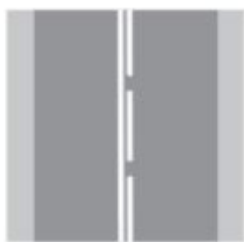
Marques longitudinals contínues adossades a discontínues
